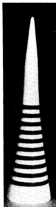
Fig. 17 Alternate disks of glass (25%) and TFE.
