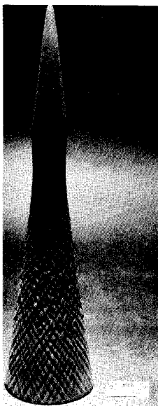
Fig. 6 Graphite (15%) filled TFE.
